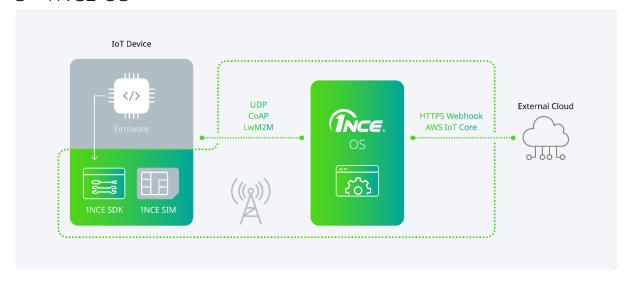
1NCE OS provides software tools to develop and manage IoT devices. These tools support in integrating the application layer on top of the network layer, which is provided by 1NCE Connect (see section 2).
